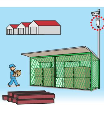
Use to activate lighting systems for safety applications in warehouses, or for monitoring intrusion attempts from up to 11.5' (3.5m) mounting height.
