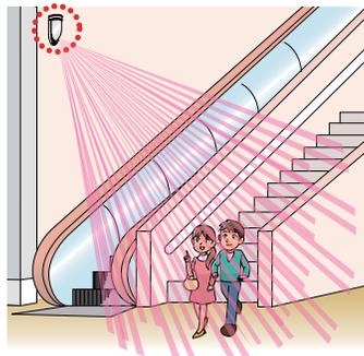
Mount up to 6m in height with a coverage of 49' (15m) x 80° 'high density mode', perfect for high installations such as open ceiling entrances.
